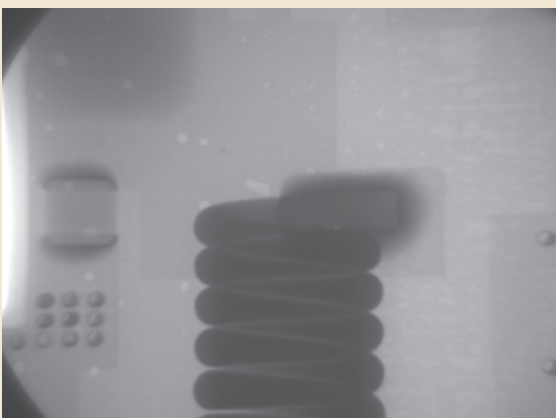
X-ray analysis confirms minimal solder voids between the PCB and copper plates.
