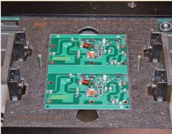
Special fixtures allow for a single reflow process.
